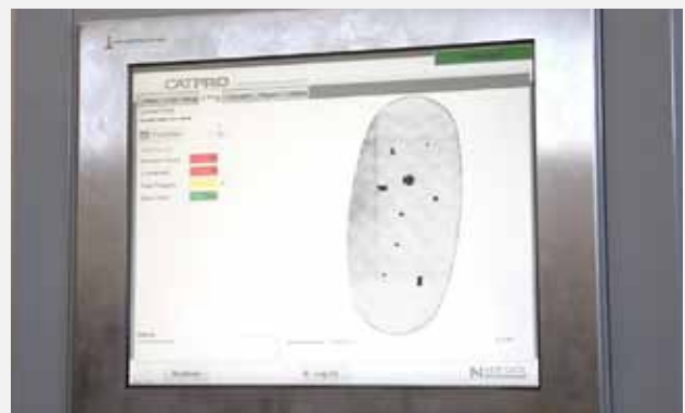
CATPRO software is recipe-driven for rapid, error-free part change-over
